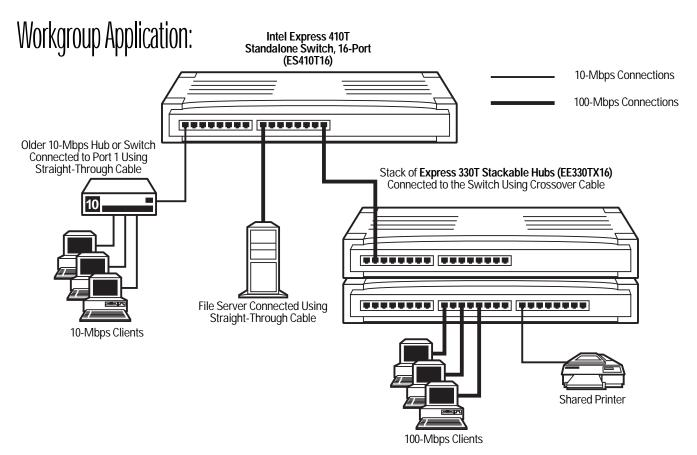
The Express 410T can serve as the backbone for a small network. Its MDI/MDI-X button allows the switch to connect to other switches and hubs using straight-through cables (instead of crossover cables).
